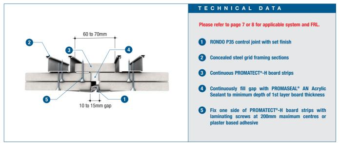
Perpendicular to steel framing (double layer)
