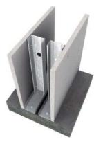
As an example, a double stud partition creating an air cavity eliminates direct mechanical connection between the surfaces. The sound transmission is reduced by breaking the sound path. In addition, the air cavity provides vibration isolation between the two sides. Sound in one room striking the one side of the wall causes it to vibrate but because of the mechanical separation and the cushioning effect of the cavity, the vibration of the other side is greatly reduced.
