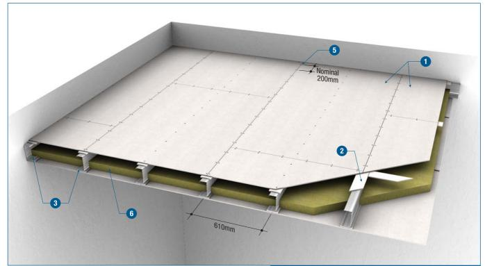
Ceiling perimeter framing at junction with masonry wall (applicable for ceiling span above 3000mm)
