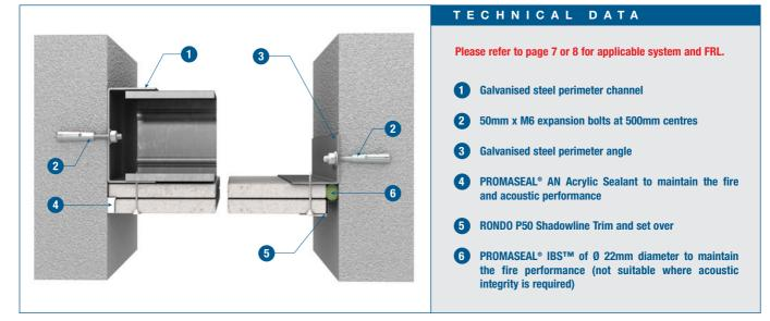
Suspended ceiling perimeter to wall intersection
